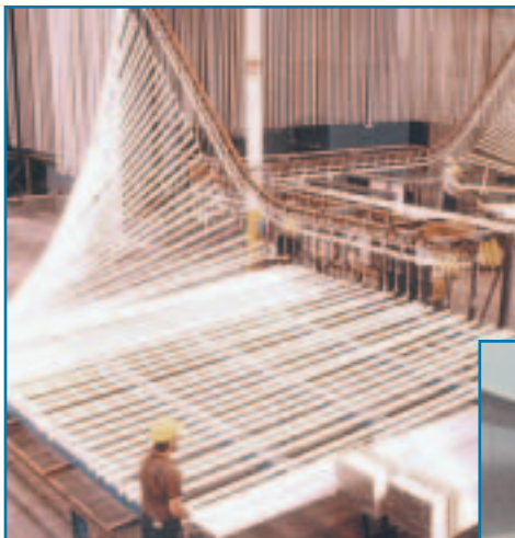
Load and unload area on a vertical paint line.
