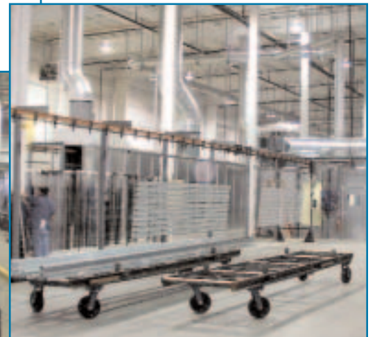
Load and unload area on a horizontal paint line.
